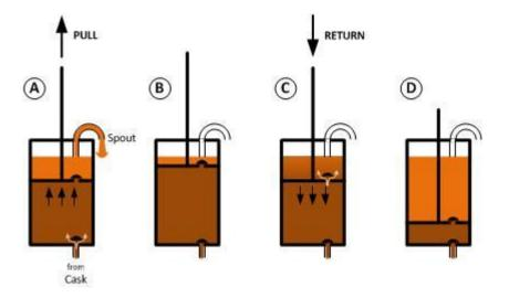
A beer hand-pump operates like an old fashioned water pump. When the handle is pulled beer is forced out of the spout from the pump cylinder, but at the same time beer is drawn from the cask to enter the cylinder, but underneath the piston (A). After a session the pump is often left in this position (B) with the cylinder full of beer hopefully sealed from the air by the one-way valves.
