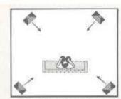
In this configuration the rear speakers may be placed slightly above the listeners and mounted on the wall for excellent coverage of the listening area. If the speakers have narrow dispersion, angle them slightly to provide for adequate coverage.
