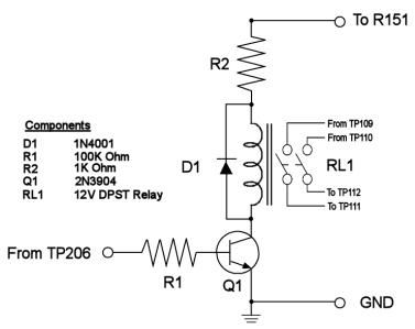
The circuit can be built on a small piece of perf board and mounted on top of the two red filter blocks using double sided sticky pads, layout is not critical. This is close to the test points, and minimises cable length. If mounted here, shielded cables are not required as noise pickup will be minimal. Power is taken from the power supply bridge rectifier end of R151, and ground from the adjacent earth tag.
