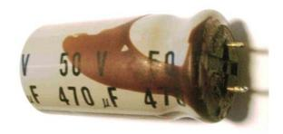
For some reason JVC decided to omit C136, one of the power supply capacitors, I would recommend fitting this, and replacing the remaining capacitors as well. The original values seemed a little low, so after careful experimentation and evaluation, I increased their values to help regulation and reduce ripple and noise. This was successful, with no noticeable increase in output voltage, but a useful decrease in ripple and noise.
