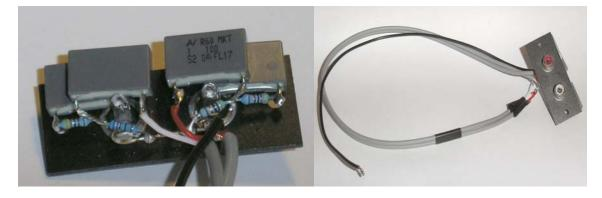
Image showing attenuator built on the back of a dual phono socket, this allows normal phono to phono leads to be used from the CD player. All connection references in the matrix balance set up will use RED or WHITE, these being the colours used in the attenuator shielded cable.
