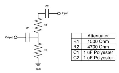
Two attenuators are required, and with the values shown they will have a voltage attenuation of approximately 12dB. It would also be possible to reduce the level recorded on to CD, but the attenuator gives added isolation and is to be recommended.
