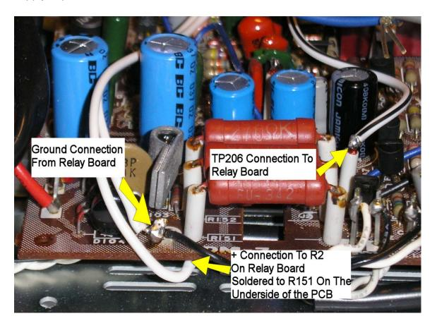
Image showing the completed relay board wired in circuit as described. This is a prototype board and looks untidy, but it worked very well. Normal hook up wire was used for all connections, hum and noise was not a problem.
