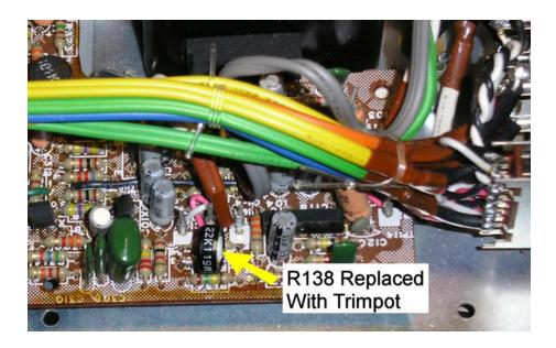
That concludes the balance adjustment. Remove attenuator cables and reassemble the demodulator.
