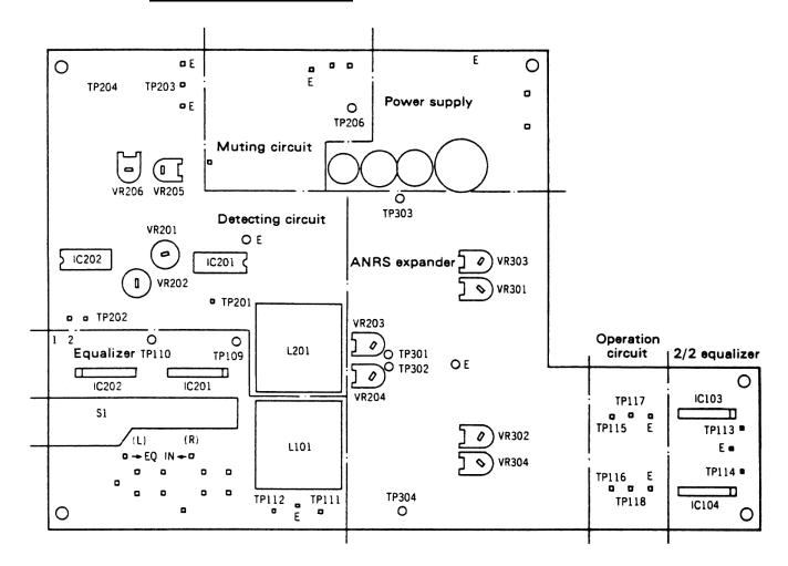
This image shows all test points and adjustment points that are required for modifying and setting up the demodulator, please refer to the service manual for full schematic information.
