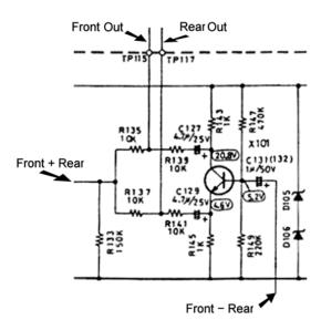
I found that when setting up my demodulator as normal, the best front to rear separation did not coincide with the best rear null point. Upon investigating this, I discovered an imbalance in the resistive mixer, showing itself as an increase in breakthrough from rear to front, and a loss of separation. This is probably caused by tolerances in the resistors making up the circuit, or simply drift with age.
