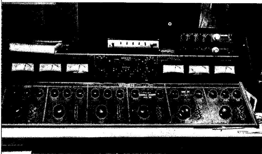
Figs. 6 and 7. Mixing console in Symphony Hall (above) is of excellent audio quality, but for use in quadraphonics engineers must devise additional versatility for it. At right, part of the monitoring equipment.
