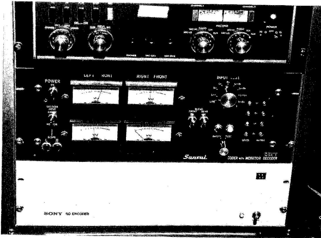
Fig. 5. Matrix encoders enable a partially recoverable four-channel signal to be impressed onto two channels for distribution and broadcast. Decoders are needed at listening end to re-create quadrasonic effect.
