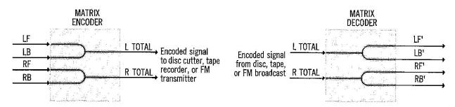
This is the basic plan of a matrix coding system for placing four sound paths onto a two-channel medium, and then recovering the four during playback. Recovered audio signals are designated with the notation (1) to emphasize that they are not exact electrical replicas of the four original, discrete signals fed into the decoder. However, in the best matrix systems, the loss (generally a few dB of channel separation) is negligible.
