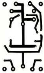
Fig. 4. Etching and drilling guide (above) and component layout for power supply (right)
