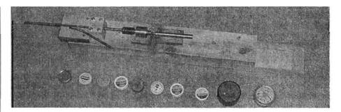
that could be *loaded from the breech*. I decided I would make a new, smooth bore, .177 caliber barrel with the nipple mounted inline into the breech; smoothbore to reduce friction, and .177 to minimize pellet weight.
