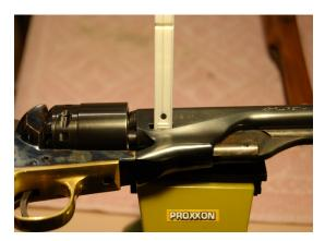
Once the wedge is removed, you can begin the honing (filing) down process on the left side (pressure side which comes in contact with the arbor ) of the wedge with a honing file or fine-tooth file.
