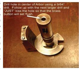
Take the Dillon Locator Button and see that it will seat fully into the hole that you just drilled in the arbor. The leg of the Locator Button will protrude in the Wedge slot.
