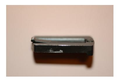
Notice that the wedge retention spring is curved upward towards the lip of the spring. Be sure this curvature remains intact at all times. Do not try to straighten the spring as that will cause the lip to not engage the barrel frame and it will become insecure.
